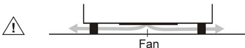
Fig. 2. Location of power supply fan DECADE II.
