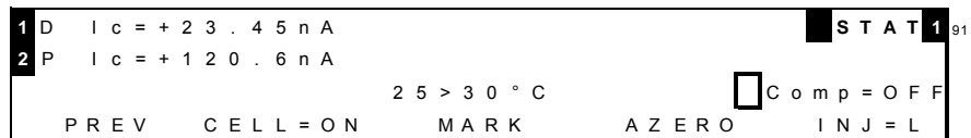
Fig. 15. DECADE II main menu (top) with active cell indicator in top right corner. Multi-STAT screen showing cell 1 (DC mode) and cell 2 (PULSE mode).
