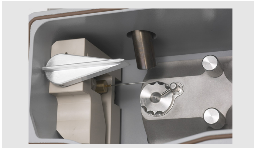
Fig. 31 View of the corona pin in the operational position for the APCI mode
