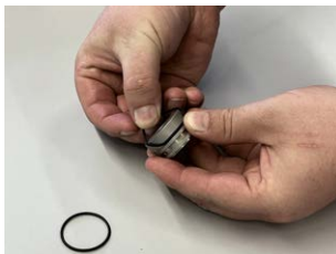
Fig. 39: Attaching the first o-ring to the seal holder
