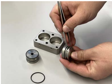
Fig. 22: Removing the o-rings from the seal holders
