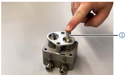
Fig. 57: Inserting the second piston rod
