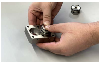
Fig. 42: Reinserting the seal holder into the pressure plate by hand
