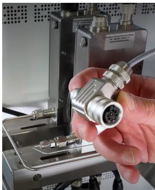
Fig. 14: Data cable of the flowmeters
