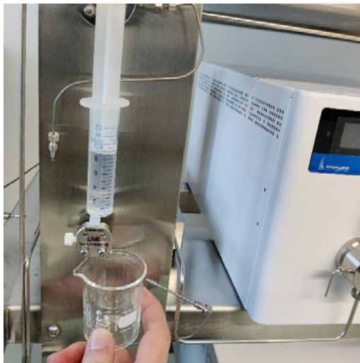
Fig. 16: Manual cleaning of the IJM
